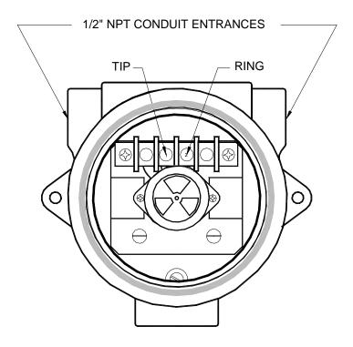
Figure 2 - Electrical Connections
